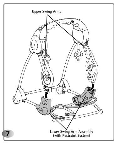
• Fit the lower swing arm assembly to the **out**side of each upper swing arm.
